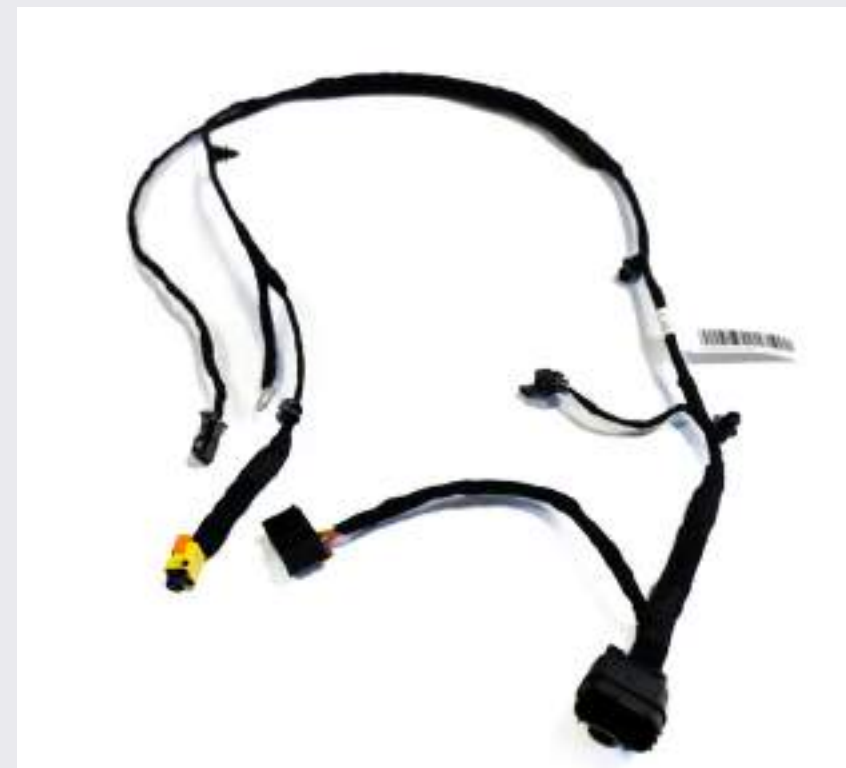
WIRING AIR BAG AND SIDE BAG
